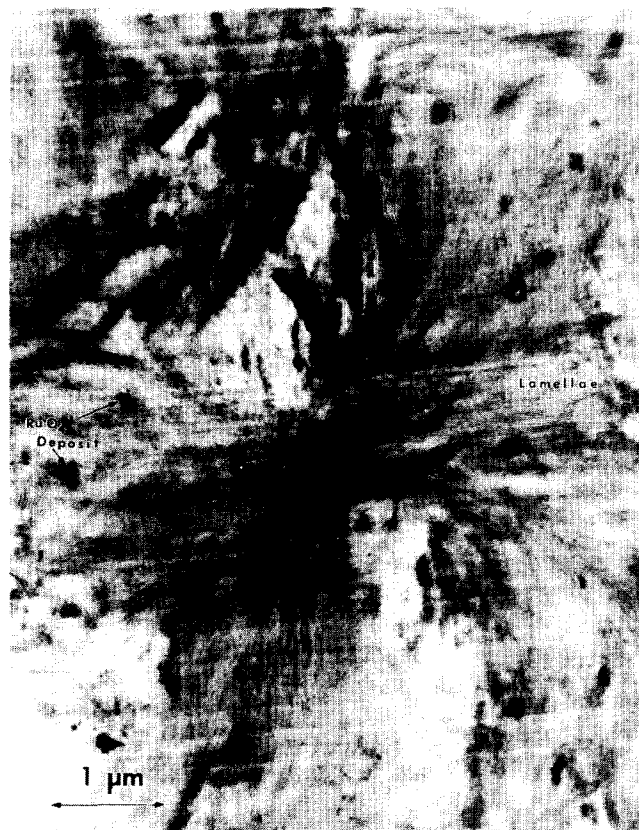
Figure 4 Transmission electron micrograph of injection moulded s-PS. Thin sections stained with ruthenium tetroxide vapour
